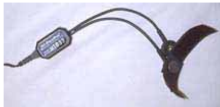
Figure 4. The Galvanic Skin Response Sensor (Picard, 2009)
